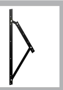
A complete range of 4-bar friction hinges (stays) providing support and control for commercial weight projected top hung (PTH) and projected side hung (PSH) sashes. The HD6 series friction stays are manufactured from aluminium and has no sliding channels.
